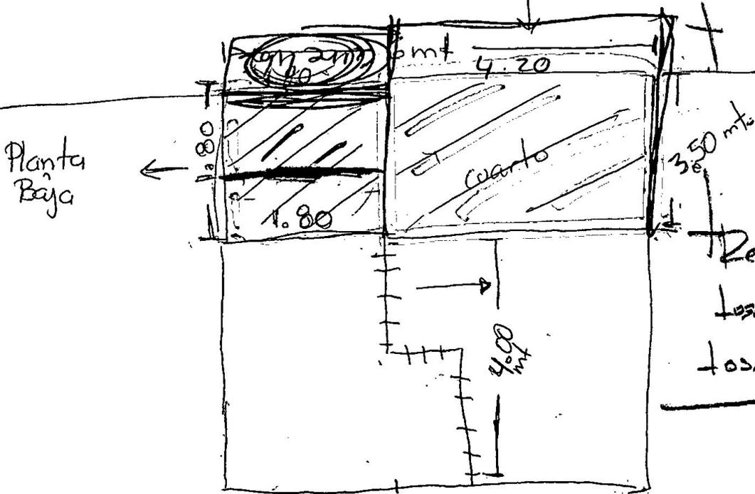
$$\begin{aligned} \text{Rec. } 4.20 \times 3.50 &= 14.70 \\ \text{Losas E.} &= 1.80 \times 1.20 = 3.24 \\ \text{Losas P.} &= 1.80 \times 1.80 = 3.24 \\ \hline &29.40 \text{ m}^2 \end{aligned}$$
